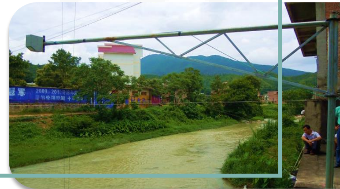
Measuring water flows without touching the water (RQ-30) in Sichuan province 非接触式测流 (RQ-30), 四川
