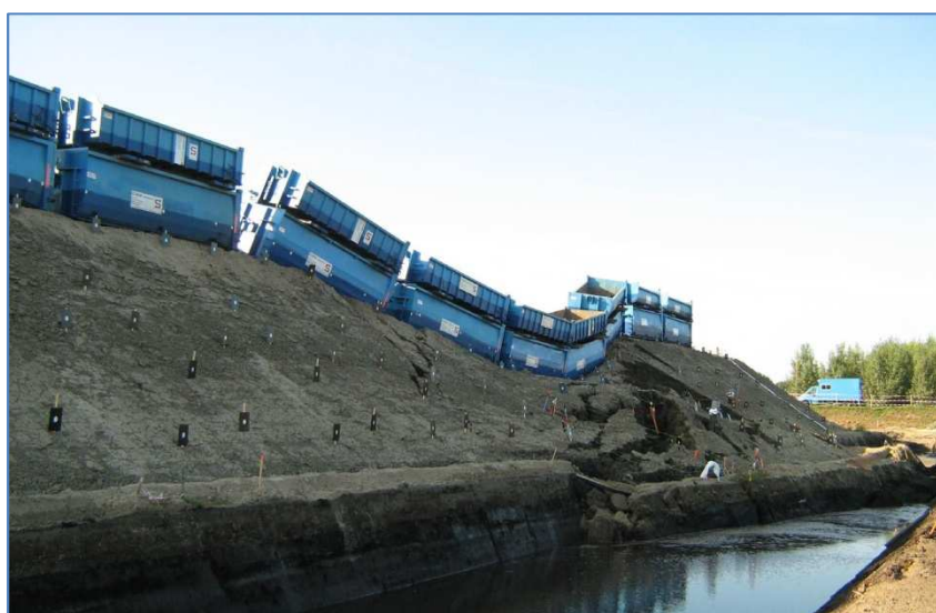
Figure 7 IJkdijk collapse experiment (2008)
